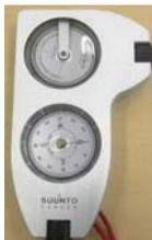
Compass and inclinometer
